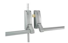
All panic hardware installations use a horizontal 'push or touch bar' that covers at least 60% of the door's width. This operating bar is used to activate a rim latch. The top and bottom latches of the **panic exit hardware** are engaged by solid rods connected to the operating bar.
