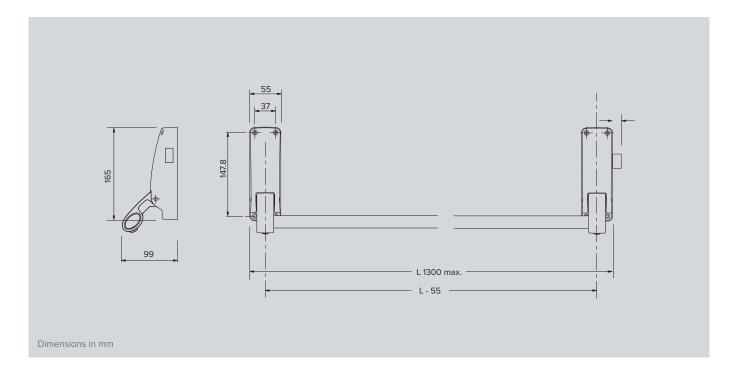
Minimum width of stiles 78mm for 13mm rebates and 90mm for 25mm rebates. For doors with less than 665mm clear opening width please seek advice from Technical Support on 0800 834102.
