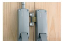
**378DDS - Double door strike** For use on double rebated doors with a rim panic latch on the first opening leaf and a vertical bolt on the second opening leaf.
