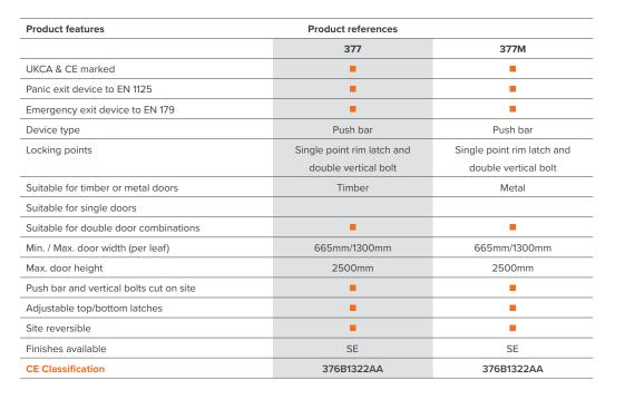
ADDITIONAL OPTIONS 370PLTM Pullman Kit 376/1021 Dogging End Box 380/1011 Alarm End Box 376.ELTS Extra Long Shoot Bolts 376FFKP Flush Face Keeper Plate
